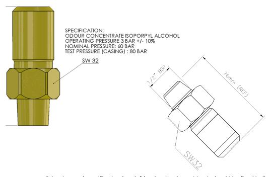
Odouriser and specification (top left), odouriser in position it should be fixed in (bottom right)
